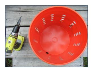
2. The lower portion of the bucket has only one opening. This is the water reservoir. You will drill one hole at the very bottom for your fill hose fitting. Insert the rubber grommet into this opening and it must fit tight or it will leak. Using your ¾ inch step drill you will want to stop before reaching the top step keeping the hole about 11/16 inches in diameter for a snug fit.
